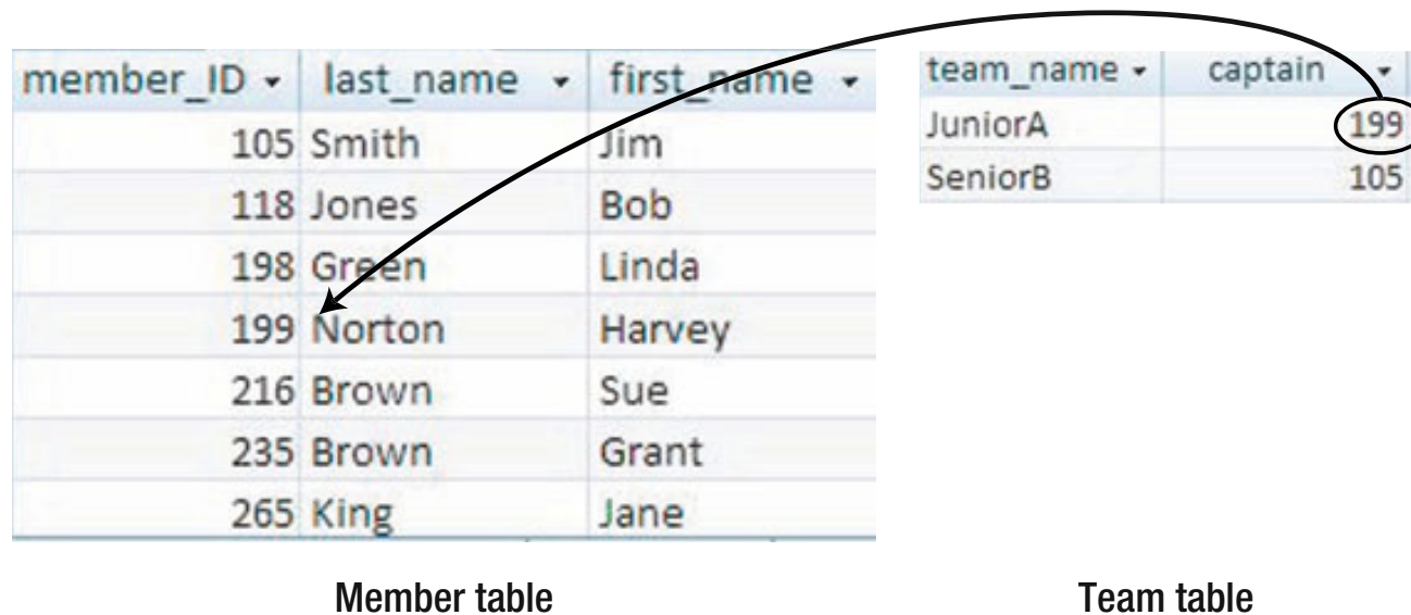
Figure 7-10. The Team table has a foreign key field (captain) referring to the Member table.
